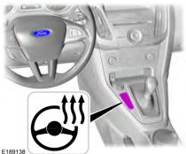
Press the button to switch the system on. The LED on the switch illuminates when the system is on.
