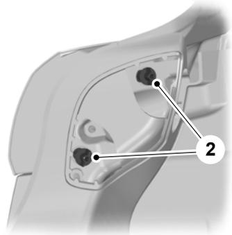
2. Remove the wing nuts and detach the clip.
