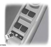
Press the control to lock or unlock the rear window controls. It lights when the rear window controls lock.
