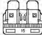
If electrical components in the vehicle are not working, a fuse may have blown. Blown fuses are identified by a broken wire within the fuse. Check the appropriate fuses before replacing any electrical components.
