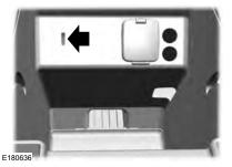
Locate your brake-shift interlock access slot. The slot is located in your center console storage bin. The access slot does not have a label.
