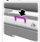
3. Locate the correct anchor on the back panel of the rear seat for the selected seating position. The anchors are labeled with the tether strap symbol and are partially covered by the gap panel. Pull the panel back to fully expose the anchors.
