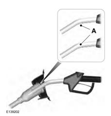
**Note:** When you insert the correct size fuel pump nozzle a spring loaded inhibitor will open. This helps to avoid refueling with the incorrect fuel.
