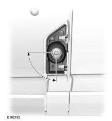
5. Operate the fuel pump nozzle within the area shown.
