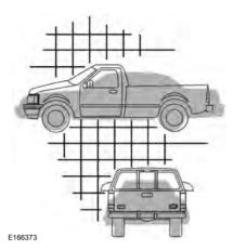
As a result of the above dimensional differences, sport-utility vehicles, vans and trucks often will have a higher center of gravity and a greater difference in center of gravity between the loaded and unloaded condition.
