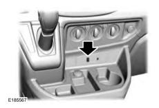
The USB port allows you to plug in media playing devices, memory sticks and charge devices (if supported). See (page 300). The extension cable must be long enough to allow the device to be safely stored while your vehicle is moving.
