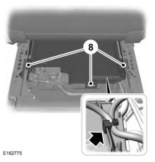
8. Remove the cable securing clips from the cover. Release the retaining clips and remove the cover.
