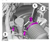
Disconnect the mass air flow sensor electrical connector and cable from the air filter cover.
