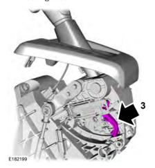
3. Locate the white lever, situated on the left hand side of the gearshift lever.
