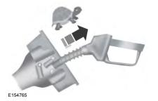
4. After you are done pumping fuel, slowly remove the fuel filler nozzle, allow about five to ten seconds after pumping fuel before removing the fuel filler nozzle. This allows residual fuel to drain back into the fuel tank and not spill onto the vehicle.
