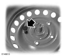
4. Remove the retaining nut to release the spare wheel bracket.
