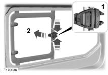
Press the unlock button to release the catch.
