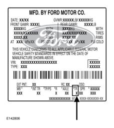
The transmission code is on the Safety Compliance Certification Label. The following table shows the transmission code along with the transmission description.
