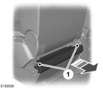
Slide the seat fully forward. Remove the cover trim by pulling up the tabs with your fingers.
