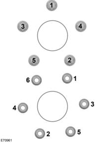
2. Install all of the lug nuts and partially tighten them in the sequence shown.
