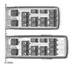
Your vehicle has LATCH lower anchors for child seat installation at the seating positions marked with the child seat symbol.
