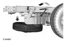
Insert the flat end of the lug wrench into the socket. Turn counterclockwise until the spare wheel rests on the ground and the cable is loose.
