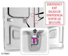
Pull the interior handle up to open the door in an emergency.
