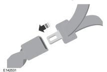
4. Insert the belt tongue into the correct buckle (the buckle closest to the direction the tongue is coming from) for that seating position until you hear a distinct click and feel the latch engage. Make sure the tongue is latched securely by pulling on it.
