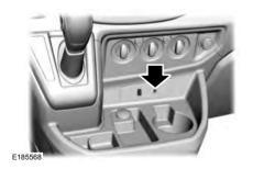
The audio input jack allows you to connect and play music from a portable music player through your vehicle speakers. You can use any portable music player designed for use with headphones. The audio extension cable must have a 0.14 in (3.5 mm) male connector at each end. The audio extension cable must be long enough to allow the portable music player to be safely stored while your vehicle is moving.
