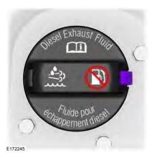
The diesel exhaust fluid tank filler neck is located below the fuel filler neck and has a blue cap. Fill the tank using a fluid pump at a diesel exhaust fluid filling station or a diesel exhaust fluid container. We recommend Motorcraft® diesel exhaust fluid, the containers are spill proof and stop the flow of fluid when the tank is full. The capacity of the diesel exhaust fluid tank is 21 liters.
