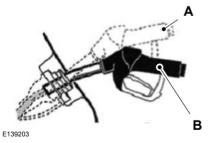
Hold the fuel pump nozzle in position B during refueling. Holding the fuel pump nozzle in position A may affect the flow of fuel and shut off the fuel pump nozzle before the fuel tank is full.
