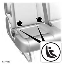
The LATCH anchors are located at the rear section of the rear seat between the cushion and seat back above the symbols as shown. Follow the child seat manufacturer's instructions to correctly install a child seat with LATCH attachments. Follow the instructions on attaching child safety seats with tether straps.
