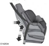
10. Before placing the child in the seat, forcibly move the seat forward and back to make sure the seat is securely held in place. To check this, grab the seat at the belt path and attempt to move it side to side and forward and back. There should be no more than 1 inch (2.5 centimeters) of movement for correct installation.
