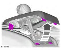
2. Use a suitable tool, for example a screwdriver, to carefully remove the housing cover.
