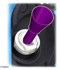
2. Insert the plastic funnel into the fuel tank filler pipe opening.
