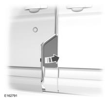
**Note:** The front door must be open before you can open and close the fuel tank filler door.
