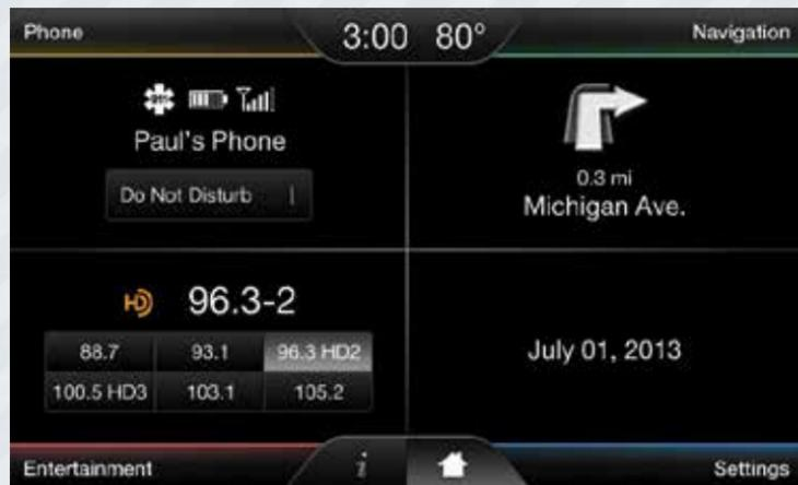
Use the four-color touchscreen to explore and interact with your vehicle. The touchscreen works the same way as traditional controls, knobs and buttons do. Press the various corners on your touchscreen to personalize the many features and settings of your vehicle all in one place. The system provides easy interaction with your cellular phone, multimedia entertainment, climate and navigation system\*.
