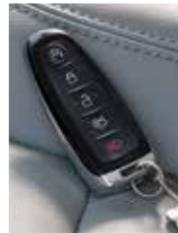
Pull a front exterior door handle to unlock and open the door. Press and hold the raised sensor on the door handle to lock your vehicle. The intelligent access transmitter also contains a mechanical key blade that you can use to unlock the driver door, if necessary. To unlock and open the liftgate, press the button on the top of the liftgate pull-cup handle.
