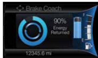
Appears after the vehicle has come to a stop. It coaches you to maximize the amount of energy returned through the regenerative braking system. The percentage displayed indicates the regenerative braking efficiency.
