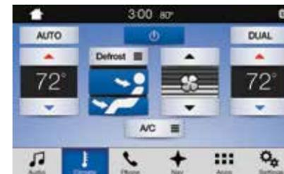
Access climate control features, including the temperature, airflow direction, fan speed and other climate features for you and your front passenger.
