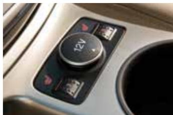
The front heated seat controls are on the center console near the gearshift lever. Rotate the dial to select your preferred heat mode.
