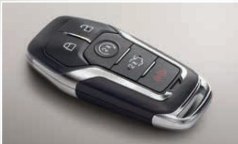
**NOTE** Your transmitter must be within 3 feet (1 meter) of the vehicle for intelligent access to function properly.
