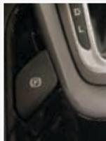
You can release the electric parking brake manually by switching the ignition on, pressing the brake pedal and then pressing the electric parking brake switch down. Refer to the **Brakes** chapter in your **Owner's Manual** for more details.
