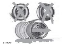
Descend a hill in the same gear you would use to climb up the hill to avoid excessive brake application and brake overheating. Do not descend in neutral; instead, disengage overdrive or manually shift to a lower gear. When descending a steep hill, avoid sudden hard braking as you could lose control. The front wheels have to be turning in order to steer the vehicle.
