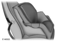
After positioning the child safety seat in the proper seating position, grasp the shoulder belt and lap belt together behind the belt tongue.
