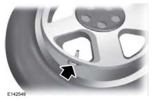
**Note:** Each road tire is equipped with a tire pressure sensor located inside the wheel and tire assembly cavity. The pressure sensor is attached to the valve stem. The pressure sensor is covered by the tire and is not visible unless the tire is removed. Take care when changing the tire to avoid damaging the sensor
