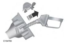
**Note:** Allow about five to ten seconds after pumping fuel before removing the fuel filler nozzle. This allows residual fuel to drain back into the fuel tank and not spill onto the vehicle.
