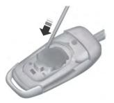
**Note:** Do not touch the battery contacts or the printed circuit board with the screwdriver.
