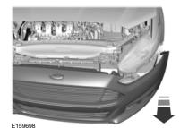
9. From the front of the vehicle, gently pull the front bumper cover forward 4 inches (10 centimeters) by grasping it next to the headlamp to be serviced and in the lower front of the wheel opening.
