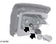
5. Remove the bulb from the bulb holder.
