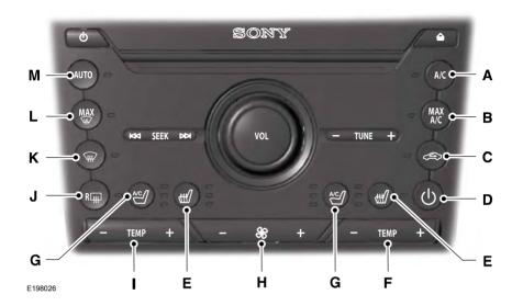
A **A/C:** Press the button to switch the air conditioning on or off. Air conditioning cools your vehicle using outside air. To improve the time to reach a comfortable temperature in hot weather, drive with the windows open until you feel cold air through the air vents.
