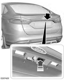
Press the release button above the license plate to unlatch the trunk. Your vehicle must be unlocked or have an intelligent access transmitter within 3 feet (1 meter) of the trunk.
