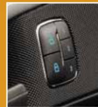
Use the memory controls on the driver's door to program and then recall memory positions. Move the seats and mirrors to the desired positions. To program up to three positions, press and hold the desired preset button until you hear a single tone. Use the controls to recall the set positions.
