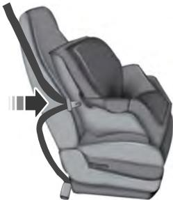
3. While holding the shoulder and lap belt portions together, route the tongue through the child restraint according to the child restraint manufacturer's instructions. Be sure the belt webbing is not twisted.
