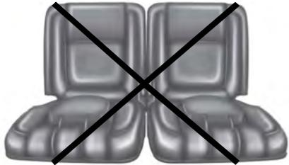
**Note:** Make sure that there are no objects such as books, purses or briefcases on the load floor before unstowing the seat. Failure to remove all objects from the top of the load floor prior to unstowing it may cause damage to the seat.
