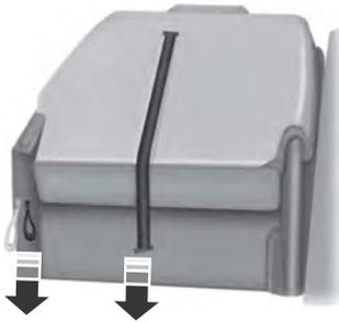
4. Release the cushion latches by pulling the short black strap while pulling on the strap located at the top of the seatback to tumble the seat all the way into the tub in the floor.
