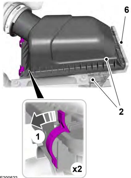
1. Remove the clips that secure the air filter housing cover.
