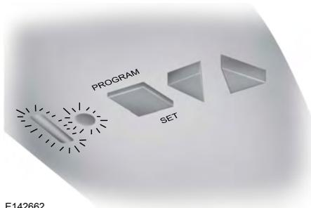
1. Press and hold the program button on the garage door opener motor until both blue indicator lights turn on.
