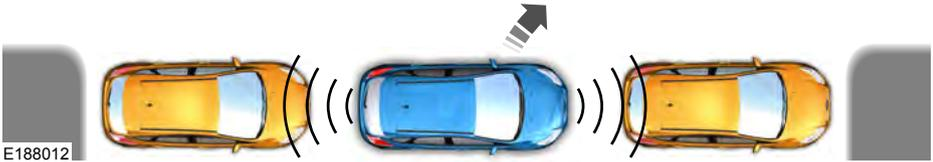
The system determines the clearance to the front and rear of your vehicle and automatically steers your vehicle out of a parallel parking space (hands-free) while you control the accelerator, gearshift and brakes. The system visually and audibly guides you to enter traffic.
