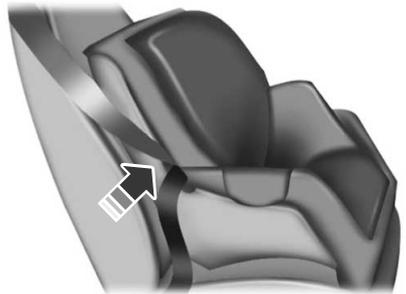
5. To put the retractor in the automatic locking mode, grasp the lap portion of the inflatable seatbelt and pull upward until you pull all of the belt out.
