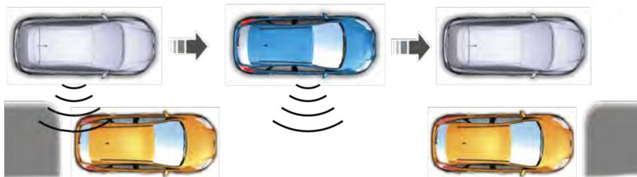
**Note:** *You can also switch the system on after you have already driven partially or completely past a parking space. Press the Active Park Assist button and the system informs you if you have recently passed a suitable parking space.*
