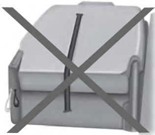
**Note:** Do not use the third row seat back as a load floor when the seatback is folded.
