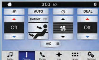
Press the **Climate** icon on the touchscreen to access climate control features, including temperature, airflow direction, fan speed and other climate features for you and your passengers.
