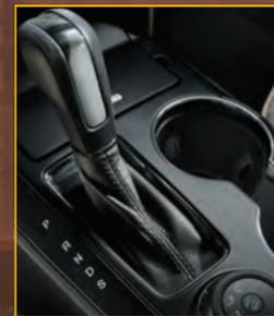
Gives you the ability to manually change gears. To use, move the gearshift lever from drive (D) to sport (S). Use the paddles on the steering wheel to change gears manually.
