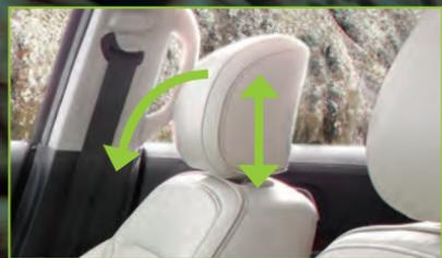
The front head restraints tilt for extra comfort. To tilt the head restraint, do the following:
