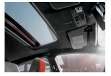
To vent the moonroof, press and hold the rear of the *TILT* control.
