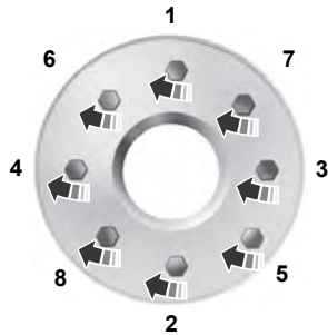
8-lug nut torque sequence
