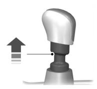
If reverse gear is not fully engaged, press the clutch pedal down and shift the gearshift lever to the neutral position. Release the clutch pedal for a moment, then raise the collar and shift the gearshift lever to reverse again.
