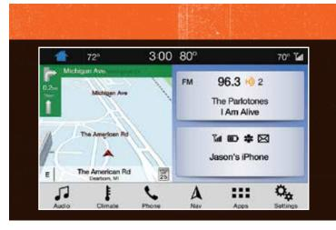
The SYNC 3 system allows you to interact with a variety of features using the touchscreen and voice commands. By integrating with your *Bluetooth* wireless technology-enabled phone, the touchscreen provides easy integration with many of your vehicle's features.
