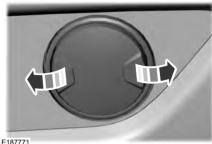
Press one side of the control to increase lower back firmness. Press the other side of the control to decrease lower back firmness.
