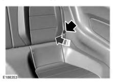
If the power decklid release does not operate because of a discharged battery, pull the rear seat left-hand side seatback cushion aside, insert the mechanical key blade into the key slot and turn the key to release the decklid latch.
