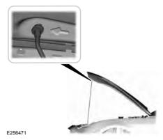
4. Open the hood. Support the hood with the strut.
