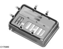
Wrap the dual purpose hose (black tube) around the channel on the bottom of the housing/casing.
