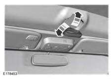
**Note:** If you keep the top open for an extended period of time or if the temperature is low, the top material may shrink slightly. If this happens, pull on the latch handle to secure the top.
