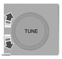
In radio mode, turn to search through the radio frequency band. In satellite radio mode, turn to find the previous or next available satellite radio station.
