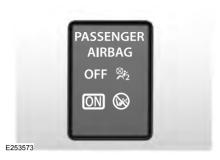
The front passenger sensing system uses a passenger airbag status indicator that illuminates indicating that the front passenger frontal airbag is either on (enabled) or off (disabled).
