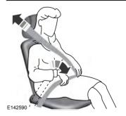
Pregnant women should always wear their seatbelt. Position the lap belt portion of a combination lap and shoulder belt low across the hips below the belly and worn as tight as comfort allows. Position the shoulder belt to cross the middle of the shoulder and the center of the chest
