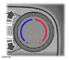
Turn the control to set the temperature.
