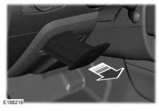
Press near the center of the door to open it. Pull out the tray.
