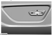
The power seat control is on the outermost side of the seat. Move the control in the direction of the arrows to raise or lower the seat cushion or to move the seat forward. backward, up or down.
