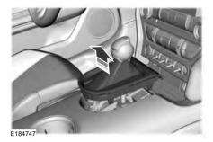
Using a flat head screwdriver or similar tool, remove the chrome bezel and gearshift bracket at the base of the gearshift lever.
