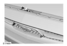
Release the hood latch by pushing the secondary release lever to your left-hand side.
