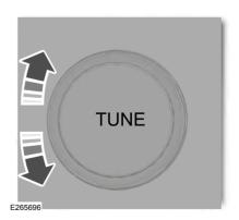
In radio mode, turn to search through the radio frequency band.
