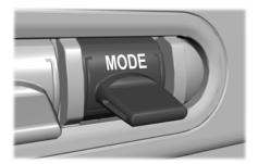
To change the drive mode setting, press the mode button on the instrument panel under the display. The first press illuminates the selected mode, subsequent presses change the selected mode.
