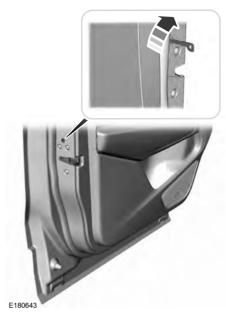
If the central locking function does not operate, lock the doors individually using the key in the position shown.
