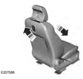
Use the seatback release to fold the back of the front seat forward for rear seat access. The release handle is on the upper back of the front seat. The seatback has memory and locks automatically in the original position.
