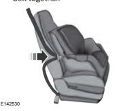
While holding the shoulder and lap belt portions together, route the tongue through the child restraint according to the child restraint manufacturer's instructions. Make sure that you have not twisted the belt webbing.
