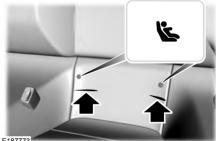
The LATCH anchors are at the rear section. of the rear seat between the cushion and seat backrest below the symbols as shown. Follow the child restraint manufacturer's instructions to properly install a child restraint with LATCH attachments. Follow the instructions on attaching child restraints with tether straps.
