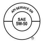
An oil that displays this symbol conforms to current engine, emission system and fuel economy performance standards of II SAC.
