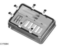
1. Unwrap the dual purpose hose (black tube) from the compressor housing.
