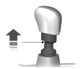
If reverse gear is not fully engaged, press the clutch pedal down and shift the gearshift lever to the neutral position. Release the clutch pedal for a moment. then raise the collar and shift the gearshift lever to reverse again.
