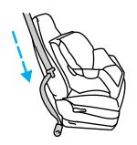
3. While holding the shoulder and lap belt portions together, route the tongue through the child seat according to the child seat manufacturer's instructions. Be sure the belt webbing is not twisted.
