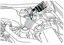
• Do not overfill the engine with oil. Oil levels above this mark may cause engine damage. If the engine is overfilled, some oil must be removed from the engine by a qualified service technician.
