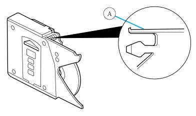
If you pull too hard on the disc holder, the disc holder may come completely out of the magazine. If this happens, reinsert the disc holder back into the magazine while pressing on the lever (A).
