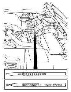
6. Wipe the indicator clean. Insert the indicator fully, then remove it again.
