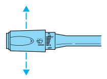
The flash rate of the turn signal will speed up considerably if the Lighting Control Module detects a left or right turn lamp bulb (front or rear) is burned out.
