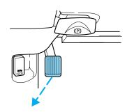
The BRAKE warning lamp in the instrument cluster illuminates and remains illuminated (when the ignition is turned ON) until the parking brake is fully released.
