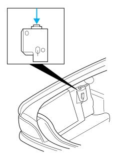
Use the following procedure to reset the fuel pump shut-off switch.
