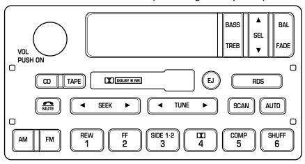
Your audio system is equipped with selective lighting, a unique lighting strategy. This lighting feature is operable when the headlamps are illuminated. During the operation of any selected mode, lighting for the individual function controls will either illuminate or turn off. Those controls which have a function for the specific mode of operation selected will be lit, while the controls which have no function for that mode will be turned off.
