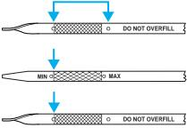
• If required, add engine oil to the engine. Refer to *Adding engine* oil in this chapter.
