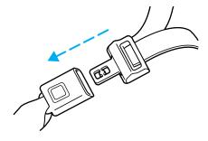
Grasp the shoulder portion and pull downward until the entire belt is extracted.
