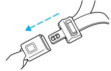
2. To unfasten, push the release button and remove the tongue from the buckle.
