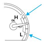
Add oil if needed (refer to *Engine oil* in the *Maintenance and care* chapter). If the oil level is correct, have your vehicle checked at your dealership or by a qualified technician.
