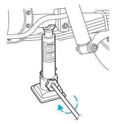
To lessen the risk of personal injury, do not put any part of your body under the vehicle while changing a tire. Do not start the engine when your vehicle is on the jack. The jack is only meant for changing the tire.
