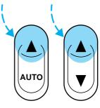
• Press the bottom portion of the rocker switch to open.
