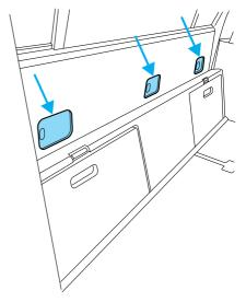
• You may need to pull the seatback forward to access the tether anchors. Make sure the seat is locked in the upright position before installing the child seat. Refer to the *Folding Down The Rear Seats* section in this chapter for information on how to operate the rear seats
