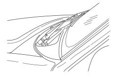
• Do not place objects over the defroster outlets. These objects can block airflow and reduce your ability to see through your windshield. Avoid placing small objects on top of the instrument panel. These objects may fall down into the defroster outlets and block airflow, in addition to damaging the climate control system.
