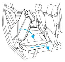
A carpeted panel will flip down from the back panel to complete the load floor.
