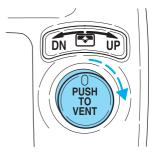
Push control once to move window (up or down) to the vent position (open approximately 2.00 inches for cab ventilation). If the window is already in the vent position and the control is pressed, no movement will occur.
