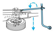
4. Remove the retainer from the center of the spare tire.
