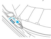
5. Push the seatback toward the front seat and completely down until it locks into place.
