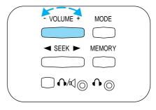
From the rear seat controls, volume control can be set no higher than the current radio setting unless the speakers are turned off. Refer to *Turning speakers on and off.*
