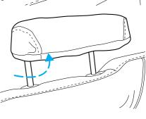
3. While holding the head restraint in "flat" position, lower the head restraint to the seat back.
