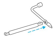
2. Insert the jack handle into the opening just above the rear bumper.
