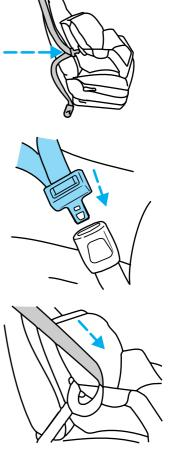
6. Allow the belt to retract. The belt will click as it retracts to indicate it is in the automatic locking mode.
