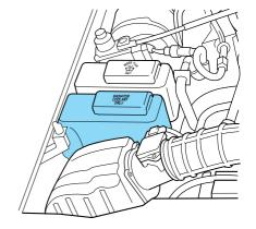
• The engine coolant should be at the "cold fill level" or within the "cold fill range" as listed on the engine coolant reservoir (depending upon application).
