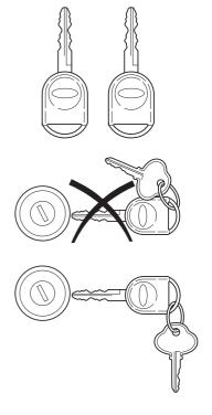
key. Check to make sure the coded key is an approved Ford coded key.
