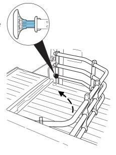
4. Evenly push down on the cargo cage and push the round knobs in on each side locking it in place.
