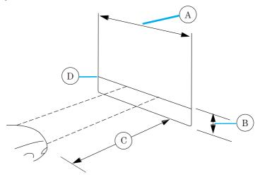
2. The center of the lamp is marked by a 3.0 mm circle on the headlamp lens. Measure the height from the center of your headlamp to the ground and mark a 2.4 meter (8 foot) long horizontal reference line on the vertical wall or screen at this height (a piece of masking tape works well).
