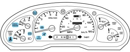
Make sure the corresponding lights illuminate or illuminate briefly. If a light fails to illuminate, have the vehicle serviced.
