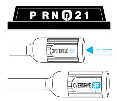
**Drive** – Not shown on the display. Activate by pressing the transmission control switch (TCS) on the end of the gearshift lever with the gearshift in the position. The TCIL (the word OFF) will illuminate on the gearshift lever. Transmission operates in gears one through three. Drive) provides more engine braking than (Overdrive) and is useful when:
