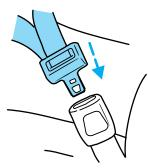
Grasp the shoulder portion and pull downward until the entire belt is extracted.
