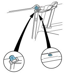
To make access to the 4th and 5th row seats easier, attach the 3rd and 4th row passenger side seat belts to the trim panel by using the snaps attached to the seat belt webbing and the trim panel.
