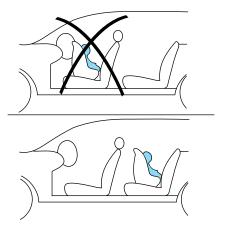
Air bags can kill or injure a child in a child seat. **NEVER** place a rear-facing child seat in front of an active air bag. If you must use a forward-facing child seat in the front seat, move the seat all the way back.
