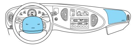
Your vehicle is equipped with a crash sensing and diagnostic module which records information about the air bag and sensor systems. In the event of a collision this module may save information related to the collision including information about the air bag system and impact severity. This information will assist Ford Motor Company in servicing the vehicle and in helping to better understand real world collisions and further improve the safety of future vehicles.
