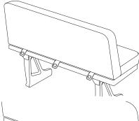
3. Clip the tether strap hook to the tether bracket mounted under rear rail of seat cushion frame.
