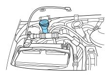
State or local regulations on volatile organic compounds may restrict the use of methanol, a common windshield washer antifreeze additive. Washer fluids containing non-methanol antifreeze agents should be used only if they provide cold weather protection without damaging the vehicle's paint finish, wiper blades or washer system.
