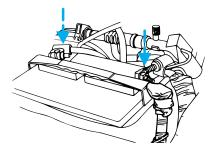
3. Unwrap the secondary positive cable and reconnect to the primary battery terminal.
