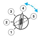
press the accelerator all the way to the floor and hold. Turn the key to the START position.
