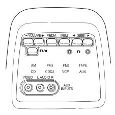
The AutoVision® controls allow the rear seat passengers to operate the radio, tape, CD or CD DJ(if equipped).
