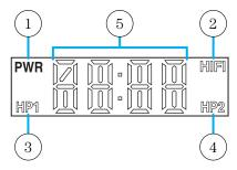
5. The **Operation indicators** illuminate when the system is powered ON, a HIFI tape is being played, or headphones are being used.
