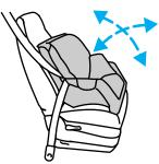
10. Try to pull the belt out of the retractor to make sure the retractor is in the automatic locking mode (you should not be able to pull more belt out). If the retractor is not locked, unbuckle the belt and repeat steps two through nine.
