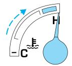
If the engine reaches a preset over-temperature condition, the engine will automatically switch to alternating cylinder operation. Each disabled cylinder acts as an air pump and cools the engine.
