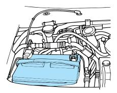
However, for severe usage or in high temperature climates and for frame mounted batteries, check the battery electrolyte level. Refer to the scheduled maintenance guide for the service interval schedules.
