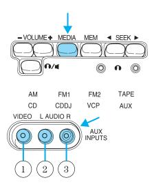
Press the MEDIA control until AUX is illuminated in the control panel. This will allow you to view the video and listen to the audio from the auxiliary input.
