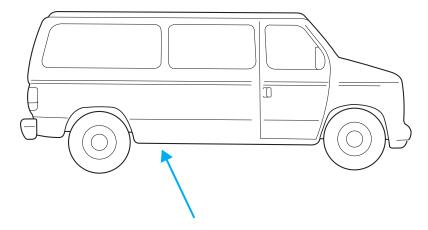
The auxiliary battery is located on the passenger side frame rail.
