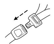
2. To unfasten, push the release button and remove the tongue from the buckle.
