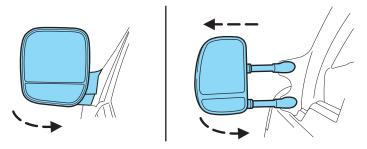
The telescoping feature (if equipped) allows the mirror to extend approximately  $76~\mathrm{mm}$  (3 inches).
