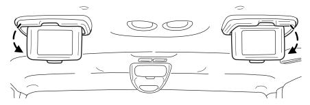
The screens rotate down to view and up into the housing to store when not in use. Ensure that the screens are latched into the housing when being stored.
