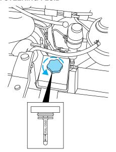
Check the fluid level when it is at ambient temperature,  $20^{\circ}$  –  $80^{\circ}$  F (-7° – 25° C):
