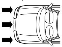
cause activation. Air bags are designed to inflate in frontal and near-frontal collisions, not rollover, side-impact, or rear-impacts unless the collision causes sufficient longitudinal deceleration.
