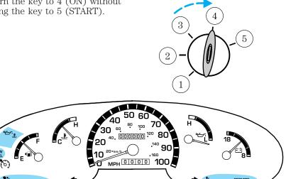
Make sure the corresponding lights illuminate or illuminate briefly. If a light fails to illuminate, have the vehicle serviced.
