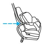
4. Insert the belt tongue into the proper buckle (the buckle closest to the direction the tongue is coming from) for that seating position until you hear a snap and feel the latch engage. Make sure the tongue is latched securely by pulling on it.
