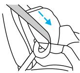
6. Allow the belt to retract. The belt will click as it retracts to indicate it is in the automatic locking mode.
