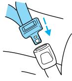
5. To put the retractor in the automatic locking mode, grasp the shoulder portion of the belt and pull downward until all of the belt is extracted.
