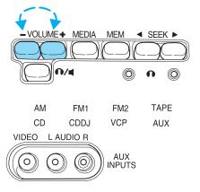
From the AutoVision® controls, the speaker volume cannot be set higher than the current volume radio setting. When in headphone mode, the AutoVision® controls can change the volume setting to any desired level.
