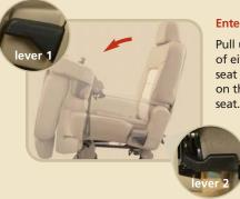
Pull up on the lever (lever 2) located at the back of the second row seat. First, the seat back will fold forward to the cushion, then
