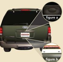
To open the liftgate glass, push the button (figure a) under the center of the license plate lamp shield.
