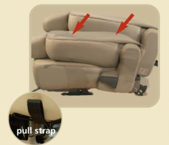
**Folding the Outboard Seats to a Load Floor Position**
