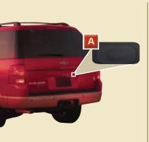
**To open the liftgate window, with** the liftgate unlocked, push the control button on the **right side** under the license plate lamp shield, or press the control on the remote entry key fob.
