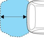
The RSS automatically turns on when the gear selector is placed in R (Reverse) and the ignition is ON. An RSS control on the instrument
