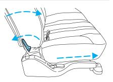
1. Pull the seat release lever located on the lower right side of the seatback while pushing the seatback down onto the seat cushion.
