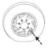
Periodically inspect the tire treads and remove stones, nails, glass or other objects that may be wedged in the tread grooves. Check for holes or cuts that may permit air leakage from the tire and make necessary repairs.
