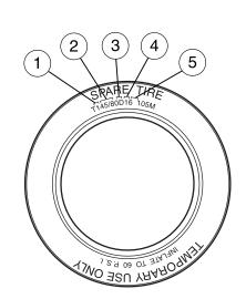
Use the recommended cold inflation pressure for optimum tire performance and wear. Under-inflation or over-inflation may cause uneven treadwear patterns.
