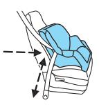
10. Try to pull the belt out of the retractor to make sure the retractor is in the automatic locking mode (you should not be able to pull more belt out). If the retractor is not locked, unbuckle the belt and repeat steps two through nine.
