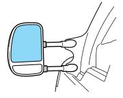
Do not remove ice from the mirrors with a scraper or attempt to readjust the mirror glass if it is frozen in place. These actions could cause damage to the glass and mirrors.
