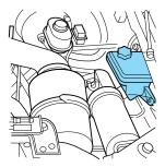
Check the fluid level when it is at ambient temperature,  $20^{\circ} - 80^{\circ}$  F (-7° - 25° C):
