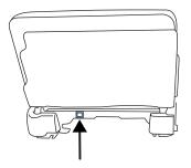
• The anchors are on the back of the seat frame.
