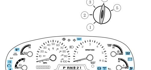
Make sure the corresponding lights illuminate or illuminate briefly. If a light fails to illuminate, have the vehicle serviced.
