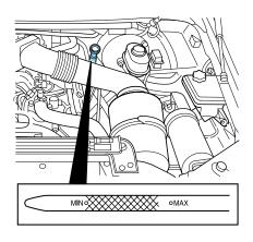
6. Wipe the indicator clean. Insert the indicator fully, then remove it again.
