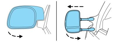
The telescoping feature (if equipped) allows the mirror to extend approximately 80 mm (3.15 inches). This feature is especially useful to the driver when towing a trailer.
