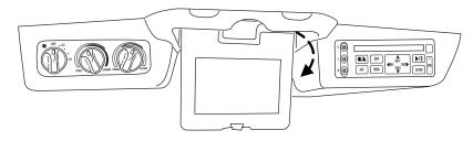
The screen rotates down to view and into the housing to store when not in use. Be sure the screen is latched into the housing when being stored.
