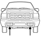
equipped with a gasoline engine have the plug exposed on the driver side of the vehicle; vehicles equipped with a Diesel engine have the plug exposed on the passenger side of the vehicle.
