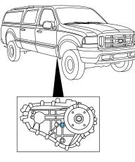
3. Add only enough fluid through the filler opening so that the fluid level is at the bottom of the opening.
