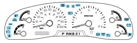
Warning lights and gauges can alert you to a vehicle condition that may become serious enough to cause expensive repairs. A warning light may illuminate when a problem exists with one of your vehicle's functions. Many lights will illuminate when you start your vehicle to make sure the bulb works. If any light remains on after starting the vehicle, have the respective system inspected immediately.
