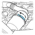
2. Carefully separate the two halves of the air filter housing.
