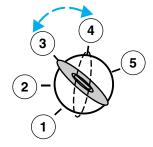
2. Turn the ignition from the 3 (OFF) position to the 4 (ON) position. Keep the ignition in the 4 (ON) position for at least one second, but no more than 10 seconds.
