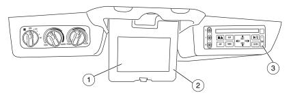
1. 7.0" (diagonal) active matrix liquid crystal display (LCD) screen.
