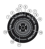
7. **H:** Indicates the tire's speed rating. The speed rating denotes the speed at which a tire is designed to be driven for extended periods of time under a standard condition of load and inflation pressure. The tires on your vehicle may operate at different conditions for load and inflation pressure. These speed ratings may need to be adjusted for the difference in conditions. The ratings range from 159 km/h (99 mph) to 299 km/h (186 mph). These ratings are listed in the following chart.
