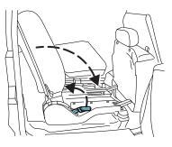
6. For bench seats only, lift up flap on seatback to release closeout panel.
