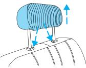
3. The headrest must be removed in order to fold the seatback down. Remove 2nd row seat headrest by pushing in both tabs while pulling up on headrest simultaneously.
