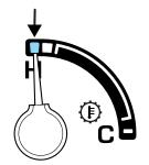
If the gauge is operating in the Yellow or Red area, stop the vehicle and verify the airflow is not restricted such as snow or debris blocking airflow through the grill. If the gauge continues to show high temperatures, see your Ford dealer.
