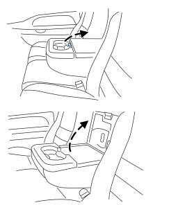
To gain access to the storage compartment in your armrest, lift the latch to open the lid. The lid cannot be opened in the upright position.
