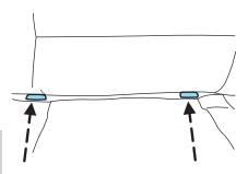
If you install a child seat with rigid LATCH attachments, do not tighten the tether strap enough to lift the child seat off the vehicle seat cushion when the child is seated in it. Keep the tether strap just snug without lifting the front of the child seat. Keeping the child seat just touching the vehicle seat gives the best protection in a severe crash.
