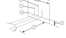
or cross marker) or on the bulb shield, internal to the lamp (mark or feature). Measure the height from the center of your headlamp to the ground (2) and mark an 8 foot (2.4 meter) long horizontal line on the wall or screen (1) at this height (masking tape works well).
