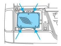
To install the new bulb, follow the removal procedures in reverse order.
