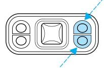
Press the control to move the seat forward, backward, up or down.
