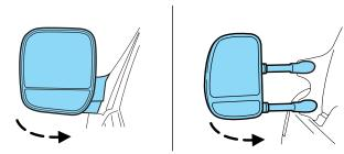
The telescoping feature (if equipped) allows the mirror to extend approximately 3.15 inches (80 mm). This feature is especially useful to the driver when towing a trailer.
