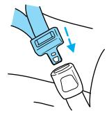
5. To put the retractor in the automatic locking mode, grasp the shoulder portion of the belt and pull downward until all of the belt is extracted.
