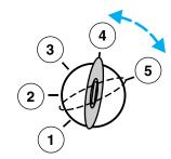
**Note:** If the engine does not start within five seconds on the first try, turn the key to 3 (OFF), wait 10 seconds and try again. If the engine still fails to start, press the accelerator to the floor and try again; this will allow the engine to crank with the fuel shut off in case the engine is flooded with fuel.
