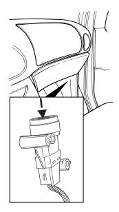
On commercial stripped chassis vehicles, this switch is located on a bracket above the brake pedal.
