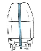
4. Clip the tether strap hook to the seat pedestal to the location shown.
