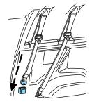
2. Pull the LH/RH seat latch handles (located under the seat) rearward to release the latch hook ends from the front strikers.
