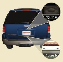
To lower the liftgate glass, push the button (figure a) under the center of the license plate lamp shield.
