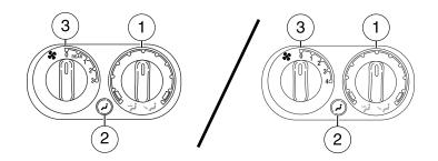
1. Temperature control: Determines temperature level. If the main climate control system is cooling in MAX A/C or  $\langle \Box \rangle$  mode, the auxiliary controls will not function as the entire vehicle will operate at a full cool temperature.
