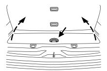
1. Open the cover from the carpeting on cargo floor to expose the winch drive nut.
