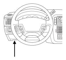
To remove a fuse use the fuse puller tool provided on the fuse panel box.
