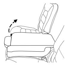
Before returning the seatback to its original position, make sure that cargo or any objects are not trapped behind the seatback. After returning the seatback to its original position, pull on the seatback to ensure that it has fully latched. An unlatched seat may become dangerous in the event of a sudden stop or collision.
