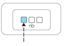
4. The indicator light will flash slowly and then rapidly. Release both buttons when the indicator light flashes rapidly. (The rapid flashing light indicates acceptance of the hand-held transmitters' radio frequency signals.)
