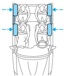
The Safety Canopy<sup>(10)</sup> is mounted to the roof side-rail sheet metal, behind the headliner, above the first and second row seats. In certain lateral collisions or rollover events, the Safety Canopy<sup>(10)</sup> system will be activated, regardless of which seats are occupied. The Safety Canopy<sup>(10)</sup> is designed to inflate between the side window area and occupants to further enhance protection provided in side impact collisions and rollover events.
