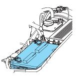
However, for severe usage or in high temperature climates, check the battery electrolyte level. Refer to *scheduled maintenance information* for the service interval schedules.
