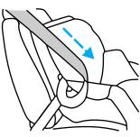
7. Pull the lap belt portion across the child seat toward the buckle and pull up on the shoulder belt while pushing down with your knee on the child seat.
