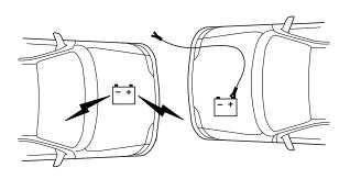
4. Remove the jumper cable from the positive (+) terminal of the disabled vehicle's battery.
