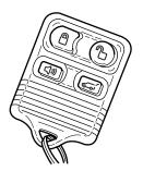
The remote entry lock/unlock feature operates in any ignition position. The liftgate glass feature operates as long as the vehicle's speed is less than 3 mph (5 km/h). The panic feature operates with the key in the 1 (OFF/LOCK) or 2 (ACC) position.
