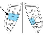
• Use the accelerator pedal to get to the desired speed. When the vehicle reaches that speed press and release the SET + control.
