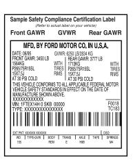
Exceeding the Safety Compliance Certification Label vehicle weight rating limits could result in substandard vehicle handling or performance, engine, transmission and/or structural damage, serious damage to the vehicle, loss of control and personal injury.
