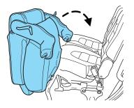
4. Bring the seat back to an upright position. The seatback should lock into position.
