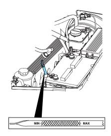
6. Wipe the indicator clean. Insert the indicator fully, then remove it again.
