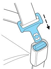
• Grasp the shoulder portion and pull downward until the entire belt is pulled out.
