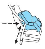
10. Try to pull the belt out of the retractor to make sure the retractor is in the automatic locking mode (you should not be able to pull more belt out). If the retractor is not locked, unbuckle the belt and repeat Steps 2 through 9.
