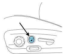
The heated seat icon in the Dual Automatic Temperature Control (DATC) will illuminate when activated.
