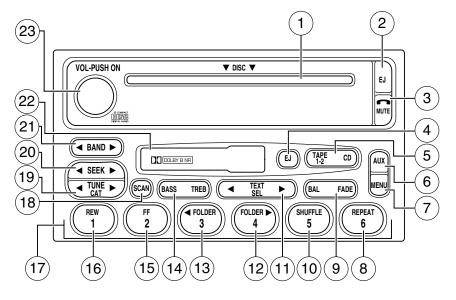
1. **CD slot:** Insert a CD with the label side up.
