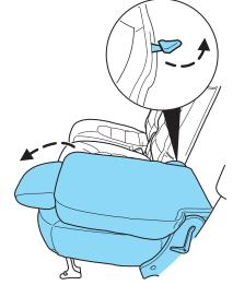
Always latch the vehicle seat to the floor, whether the seat is occupied or empty. If not latched, the seat may cause injury during a sudden stop.
