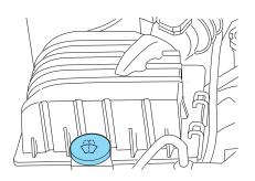
Only use a washer fluid that meets Ford specification WSB-M8B16–A2. Refer to *Lubricant specifications* later in this chapter.
