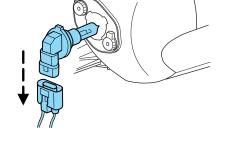
Handle a halogen headlamp bulb carefully and keep out of children's reach. Grasp the bulb only by its plastic base and do not touch the glass. The oil from your hand could cause the bulb to break the next time the headlamps are operated.
