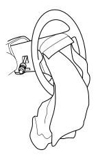
If the airbag has deployed, **the airbag will not function again and must be replaced immediately.** If the airbag is not replaced, the unrepaired area will increase the risk of injury in a collision.
