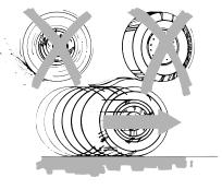
roll and if they aren't rolling, you won't be able to steer. The front wheels have to be rolling in order to steer the vehicle. Rapid pumping of the brake pedal will help you slow the vehicle and still maintain steering control. If your vehicle has four wheel anti-lock brakes, apply and hold the brakes firmly. Do not "pump" the brakes.
