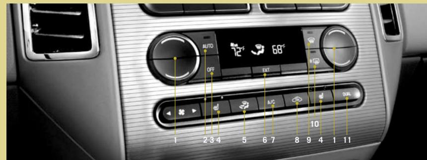
determine fan speed, airflow location, A/C (on or off) and outside or recirculated air based on your temperature selection. Press again to deactivate.
