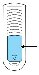
Remove the screw and unlatch the battery cover to access the batteries.
