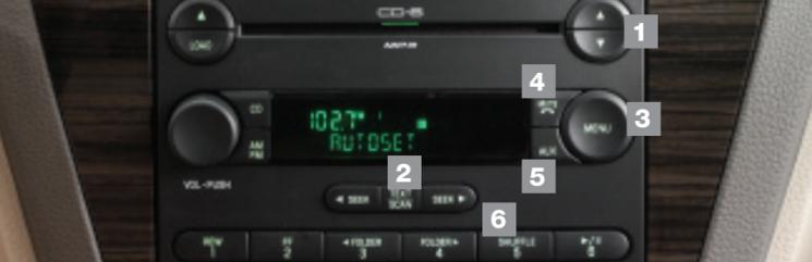
**1. TUNE/DISC SELECTOR:** Press and release to manually advance up/down the radio frequency or to access the next/previous disc. Also used to make selections within the MENU function.
