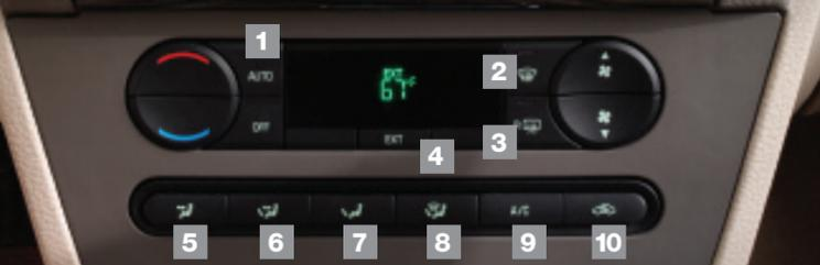
**1. AUTO:** Press to activate automatic temperature control. The system will automatically determine fan speed, airflow location, A/C (on or off) and outside or recirculated air, to heat or cool the vehicle to reach the desired temperature. Press again to deactivate.
