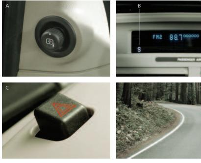
A. POWER SIDE VIEW MIRRORS – Rotate the control clockwise to adjust the right mirror, and counterclockwise to adjust the left mirror. Then move the control in the direction you wish to tilt the mirror. Return to the center position to lock the mirror in place.
