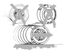
roll and if they aren't rolling, you won't be able to steer. The front wheels have to be rolling in order to steer the vehicle. Rapid pumping of the brake pedal will help you slow the vehicle and still maintain steering control. If your vehicle has four wheel anti-lock brakes, apply and hold the brakes firmly. Do not "pump" the brakes.
