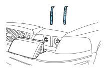
4. Disconnect the electrical connector from the bulb by pulling rearward.
