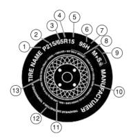
7. **H:** Indicates the tire's speed rating. The speed rating denotes the speed at which a tire is designed to be driven for extended periods of time under a standard condition of load and inflation pressure. The tires on your vehicle may operate at different conditions for load and inflation pressure. These speed ratings may need to be adjusted for the difference in conditions. The ratings range from 81 mph (130 km/h) to 186 mph (299 km/h). These ratings are listed in the following chart.
