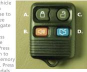
being used). Car finder Press A twice within 3 seconds. The horn will chirp and the turn lamps will flash. It is recommended that this method be used to locate your vehicle, rather than using the panic alarm. For more information regarding the memory seats/adjustable pedals/easy entry-exit feature, refer to your Owner's Guide.
