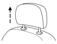
2. Press and hold the unlock/remove button, then pull up on the head restraint.
