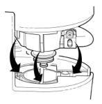
2. Once aligned, seat the sealant canister by lightly pushing down until you hear an audible click.
