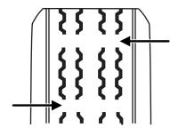
the same height as these "wear bars", the tire is worn out and must be replaced.
