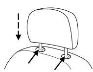
Properly adjust the head restraint so that the top of the head restraint is even with the top of your head and positioned as close as possible to the back of your head. For occupants of extremely tall stature, adjust the head restraint to its full up position.
