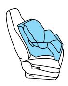
2. Pull down on the shoulder belt and then grasp the shoulder belt and lap belt together.
