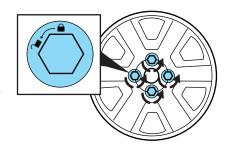
4. Loosen each wheel lug nut one-half turn counterclockwise but do not remove them until the wheel is raised off the ground.
