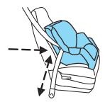
8. Check from time to time to be sure that there is no slack in the lap/shoulder belt. The shoulder belt must be snug to keep the lap belt tight during a collision.
