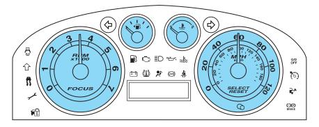
**Speedometer:** Indicates the current vehicle speed.
