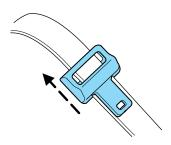
3. While holding both shoulder and lap portions next to the tongue, route the tongue and webbing through the child seat according to the child seat manufacturer's instructions. Be sure that the belt webbing is not twisted.
