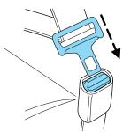
Grasp the shoulder portion and pull downward until the entire belt is pulled out.
