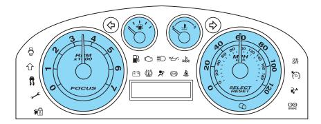
**Speedometer:** Indicates the current vehicle speed.
