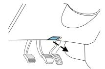
2. Go to the front of the vehicle and locate the auxiliary latch centered under the front of the hood and then release it by pushing the auxiliary latch to the left.
