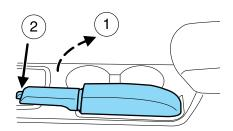
The BRAKE warning lamp will illuminate and will remain illuminated until the parking brake is released.
