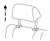
Lower the head restraint by pressing and holding the guide sleeve release button and pushing down on the head restraint.
