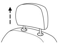
2. Simultaneously press and hold both the adjust/release button and the unlock/remove button, then pull up on the head restraint.
