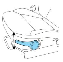
Lift the control to adjust the angle of the seatback.
