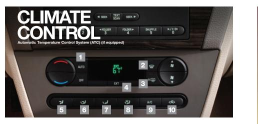
1. AUTO: Press to activate automatic temperature control. The system will automatically determine fan speed, airflow location, A/C (on or off) and outside or recirculated air, to heat or cool the vehicle to reach the desired temperature.
