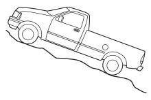
Descend a hill in the same gear you would use to climb up the hill to avoid excessive brake application and brake overheating. Do not descend in neutral. Disengage overdrive or manually shift to a lower gear. When descending a steep hill, avoid sudden hard braking as you could lose control. In a vehicle without four wheel anti-lock brakes, if you lock up the front brakes, the front wheels can't
