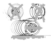
roll and if they aren't rolling, you won't be able to steer. The front wheels have to be rolling in order to steer the vehicle. Rapid pumping of the brake pedal will help you slow the vehicle and still maintain steering control. If your vehicle has four wheel anti-lock brakes, apply and hold the brakes firmly. Do not "pump" the brakes.
