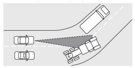
• There may be issues with the detection of vehicles in front when driving into and coming out of a bend or curve in the road.
