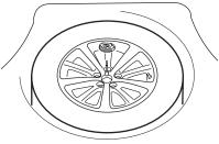
5. Safely secure the wheel by screwing the large wing nut onto the extension bolt.
