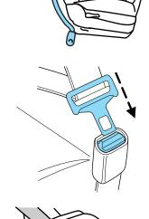
5. To put the retractor in the automatic locking mode, grasp the shoulder portion of the belt and pull downward until all of the belt is pulled out.
