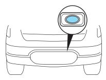
2. Press the release button located near the license plate.
