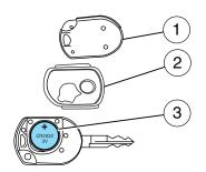
3. Remove the old battery (3). **Note:** Please refer to local regulations when disposing of transmitter batteries.
