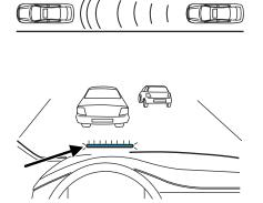
The vehicle will not stop unless the driver presses the brake pedal. If the brake pedal is pressed then braking is implemented with full brake function, even if the force on the brake pedal is light.
