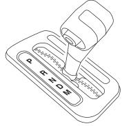
To return to normal D (Drive) position, move the shift lever back from M (Manual) to D (Drive). The transmission will operate in gears one through six.
