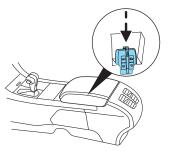
the back-up slot, located in your center console utility compartment. Insert the IA key into the slot with buttons facing out and with key ring up. After inserting the IA key into the back-up slot, use the START/STOP button and brake pedal to start your vehicle as usual. The vehicle should respond normally as long as the IA key is in the back-up slot in the center console utility compartment. Once the vehicle is started, the IA key can be removed from the back-up slot, if desired.
