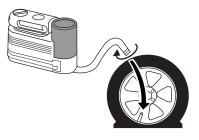
Note: When the sealing compound is first added into the tire, the air pressure gauge reading on the compressor unit may indicate a higher value; this is normal and should be no reason for concern. The pressure will drop after about 30 seconds of operation. The 300
