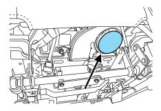
• The filter can be accessed from the 2nd row foot-well area. Move the front seats all the way to the full front and full up positions to ease access.
