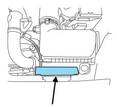
D. Remove two bolts that attach the air filter assembly to the front of the vehicle (2).
