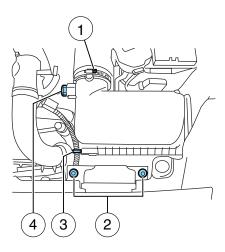
C. Remove the bolt cover (if equipped).
