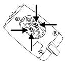
4. Snap the battery cover back onto the transmitter and install the backup key.
