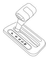
**WARNING:** Always set the parking brake fully and make sure the gearshift is latched in P (Park). Switch the ignition off and remove the key whenever you leave your vehicle.
