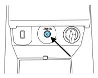
attaching your portable music device to the audio system. If your vehicle is equipped with a navigation system, refer to *Auxiliary input jack* section in the *Audio features* chapter of your *Navigation System* supplement.
