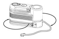
2. Press the button located on the temporary mobility kit compressor housing below the canister while pulling up on the sealant canister.
