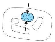
Push and hold the front of the lumbar control to increase the firmness of the selected portion of the seatback or push and hold the rear of the lumbar to decrease the firmness.
