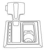
4. Insert the screwdriver (or similar tool) into the access hole and press while pulling the gearshift lever out of the P (Park) position and into the N (Neutral) position.
