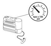
5. Turn the compressor off by pressing the on/off button.
