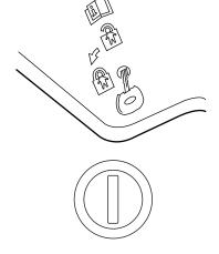
• Insert the key and turn to the unlock position (key vertical) to disengage the childproof locks.
