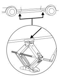
6. Lower the wheel by turning the jack handle counterclockwise.
