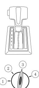
3. Turn the key to 3 (on) without turning the key to 4 (start).
