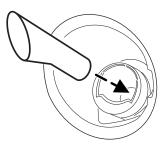
3. Fill the vehicle with fuel from the portable fuel container.
