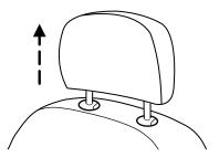
2. Simultaneously press and hold both the adjust/release button and the unlock/remove button, then pull up on the head restraint.
