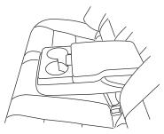
If your vehicle is equipped with cup holders and a storage compartment, they are located in the rear seat armrest. To access the cup holders, rotate armrest into use position. To open the storage compartment (if equipped), pull up on the latch.
