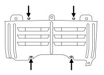
Some vehicles may be equipped with an aero-shield under the engine. This shield needs to be removed for service, including oil and filter changes. It is secured with four quick release fasteners.
