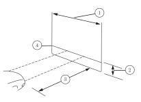
height (a piece of masking tape works well). The center of the lamp is marked by a 3 mm circle on the headlamp lens.
