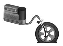
8. Inflate the tire to the pressure listed on the Tire Label located on the driver's door or the door jamb
