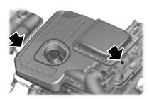
4. Remove the bolts from each side of the air cleaner assembly (A) as shown with arrows.
