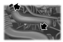
5. Install the air cleaner outlet tube (C) and tighten the hose clamps.
