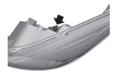
4. Locate the vertical adjuster on each headlamp. Using a Phillips #2 screwdriver, turn the adjuster either clockwise or counterclockwise in order to aim the headlamp. The horizontal edge of the brighter light should touch the horizontal reference line.
