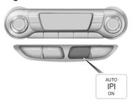
Press the button; the touch screen displays a message and a corresponding graphic to indicate it's searching for a parking space. Use the turn signal to indicate which side of the vehicle you want the system to search on.
