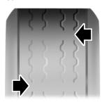
When the tread is worn down to 1/16th of an inch (2 millimeters), tires must be replaced to help prevent your vehicle from skidding and hydroplaning. Built-in treadwear indicators, or wear bars, which look like narrow strips of smooth rubber across the tread will appear on the tire when the tread is worn down to 1/16th of an inch (2 millimeters).
