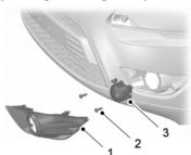
**Note:** You cannot separate the fog lamp bulb from the bulb holder.
