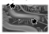
1. Loosen the hose clamps for air cleaner outlet tube (C). Disconnect the tube from the air cleaner assembly (A).
