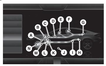
This screen displays how the electric vehicle system transfers power in order to accelerate or recharge the battery. The power flow screens show power going to or through a component. These screens are for your information only, and do not require any input from you.
