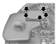
2. Install the air cleaner cover (B) and tighten the  $5~{\rm bolts.}$
