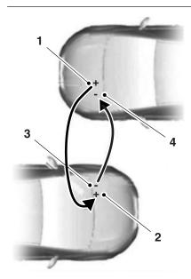
**Note:** In the illustration, the vehicle on the bottom is used to designate the assisting (boosting) battery.
