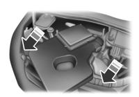
5. Lift the air cleaner assembly (A) from the mounting studs, then rotate and pull it towards the front of the vehicle.
