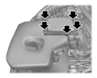
6. Loosen the 5 bolts from the air cleaner cover (B).
