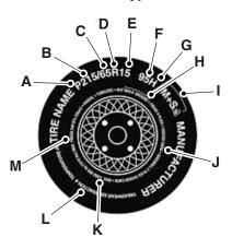
P215/65R15 95H is an example of a tire size, load index and speed rating. The definitions of these items are listed below. (Note that the tire size, load index and speed rating for your vehicle may be different from this example.)
