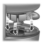
1. Align the sealant canister with the temporary mobility kit housing.
