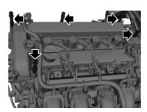
3. Position the air cleaner assembly (A) onto the engine and make sure the assembly is aligned with the studs.
