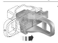
• On C-MAX Energi vehicles, slide the service disconnect handle to the right.
