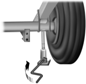
Rear axle jacking points - All models except E-350 dual rear wheel and E-450:
