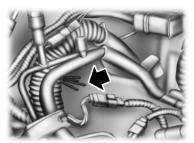
There will also be one power lead for each switch found as a blunt-cut and sealed wire located to the right of the glove box door and just above the passenger side kick panel.
