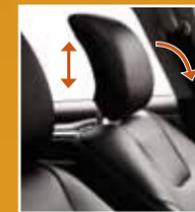
Your vehicle's front head restraints have a tilting feature for extra comfort. **To tilt the head restraint:** Adjust the seat back to an upright driving or riding position. Pivot the head restraint forward toward your head to the desired position. Once it is in the forward-most position, tilting it forward once more will release it to the upright position.
