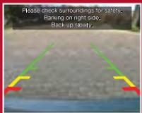
Provides a video image of the area behind the vehicle in either the rearview mirror or the display in the center of the instrument panel. The image automatically appears when the vehicle is in R (Reverse) and uses green, yellow and red guides to alert you of your proximity to objects.
