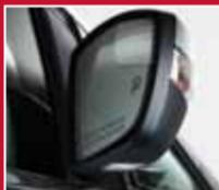
Designed to assist you by increasing the visibility along the side of your vehicle.
