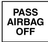
The front passenger sensing system uses a “passenger airbag off” or “pass airbag off” indicator which will illuminate and stay lit to remind you that the front passenger frontal airbag is disabled. The indicator
