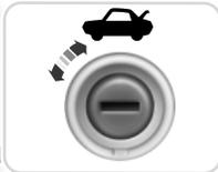
In the event of battery failure, you can open the trunk on the convertible by using your master key in the key cylinder between the seat cushion located in the back seat on the driver's side.
