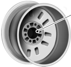
**Note:** Inspect the wheel pilot hole (1) and mounting surface prior to installation. Remove any visible corrosion or loose particles.
