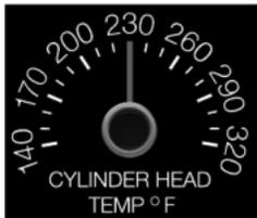
Displays the engine's cylinder head temperature.
