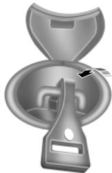
4. Clip the tether strap to the anchor as shown.
