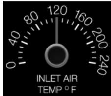
Displays the temperature of the air in the cold air inlet tube.
