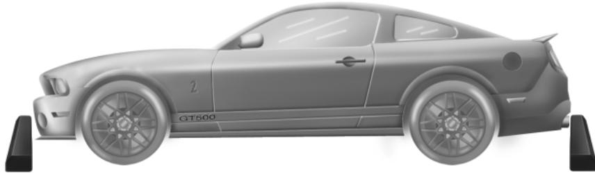
Your vehicle is designed for high speed capability and has been aerodynamically tuned to reach 200 mph (322 km/h) when properly equipped. Some of the aerodynamic tuning has been achieved with the lower front air dam, which is attached below the front splitter. The lower front air dam is removable with basic tools to suit your driving conditions, especially if they include steep driveway angles, rough roads, high curbs or harsh climates.
