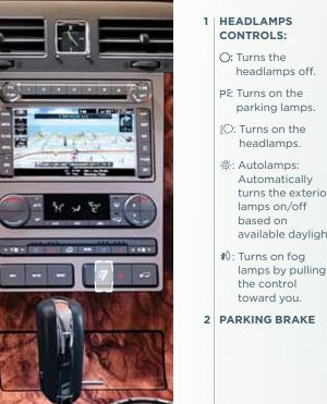
**3 MULTI-FUNCTION**/ headlamps off. P€: Turns on the parking lamps. D: Turns on the headlamps. -&-: Autolamps: Automatically turns the exterior lamps on/off based on available daylight. ŧ): Turns on foa
