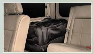
**POWERFOLD**\* **THIRD-ROW SEAT**\*: 60/40 split-folding bench seat uses a power-activated seat back release. Fold one side down or both for more flexibility.
