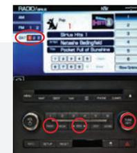
**TIP** Touch the **SHOW OPTIONS** button on the bottom right of the screen if **SCAN** and **DIRECT TUNE** are not present.
