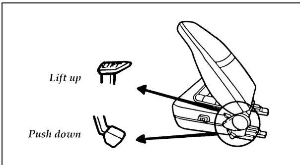
Prior to operating the vehicle, check to ensure that the seat assembly is locked by pushing or pulling the seat forward or rearward. If seat does not lock, repeat steps 2 and 3.
