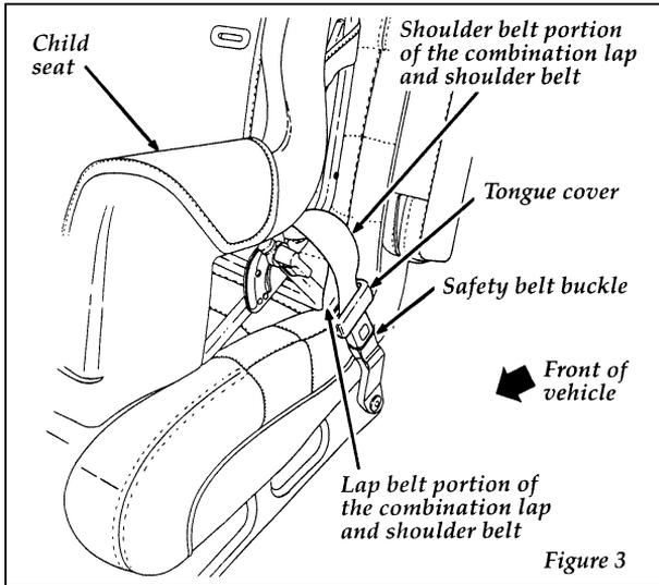
6. Push down on the child seat and pull up on the shoulder belt portion to tighten the lap belt portion of the combination lap and shoulder belt. See Figure 4.
