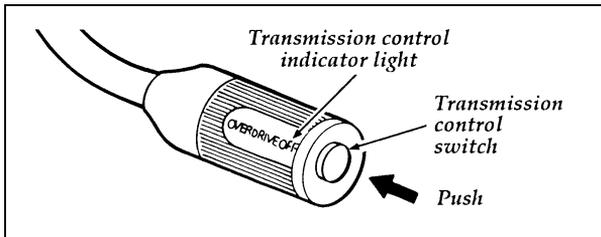
**Transmission Control Switch and indicator light (located on the gearshift lever)**
