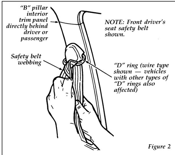
2. Rotate and fold the belt webbing over itself as required to remove the twist.
