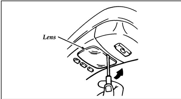
To remove the bulbs, use a screwdriver or coin to push up and rotate counterclockwise 90°. The bulb and bulb holder will then drop out from the lamp as shown:
