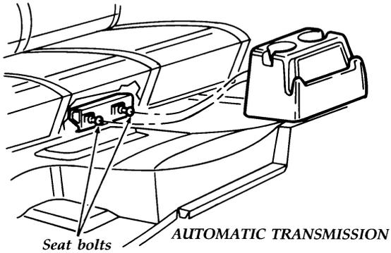
*NOTE: Consoles may be removed from seat bolts for cleaning and emptying.*
