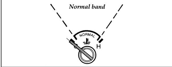
Engine coolant temperature gauge
