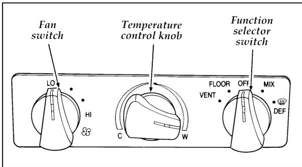
To turn your Heater system on, select any position except OFF. This will turn the fan ON and allow air flow into the vehicle. Select OFF to turn your Heater off. This will turn the fan off and stop outside air from coming into the vehicle.
