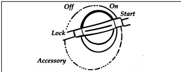
The positions of the key in the ignition lock cylinder.
